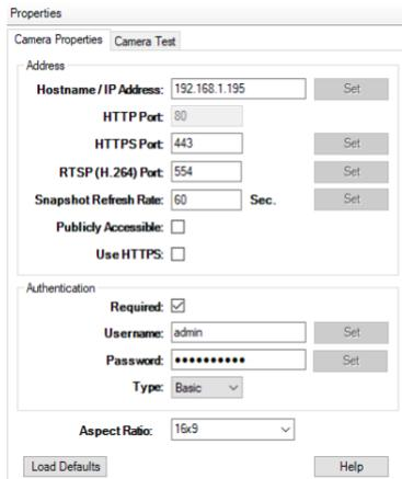
5. Confirm the camera is successfully connected by viewing the Properties tab under Advanced Properties in Composer Pro. The Camera’s Model, Firmware, and Serial Number fields will be populated.
