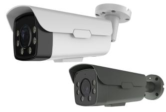
The 8MP ClareVision Bullet camera includes a Sony<sup>®</sup> Starvis<sup>™</sup> image sensor with a 2.7-13.5 mm motorized varifocal lens that supports autofocus. The enables IR night vision up to 60 meters, and supports smart detection capabilities such as human body detection, line crossing, loitering, intrusion, and people gather. The camera can be used standalone with an SD card or NVR, as well as accessed through a ClareOne or Control4 system.
